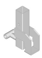
The VT Sheet Pile Clamp is placed on sheet pile profiles or trench sheets from 5-15 mm and fastened. It is easy to install thanks to the integrated DW15 nut and the locking thread.
