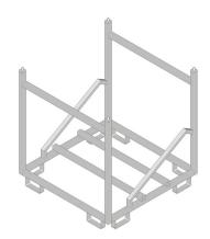
Depending on the type of barrier, between 45 and 60 barriers can be transported.
