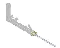
The VT Steelflange is used to hold an edge protection post on steel beams without having to drill for it. This clamp allows clamping widths of 80-460 mm.
