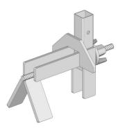
This clamp is used to attach standard edge protection to sheet pile profiles, trench shoring panels and HEB beams. Clamping width up to 150 mm and easy to mount. Tightening using a hammer.
