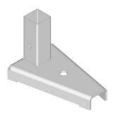
The VT Foot is used to hold an edge protection post on all flat surfaces, e.g. in-situ concrete ceilings. This horizontal attachment can be fastened with various screws and anchors.
